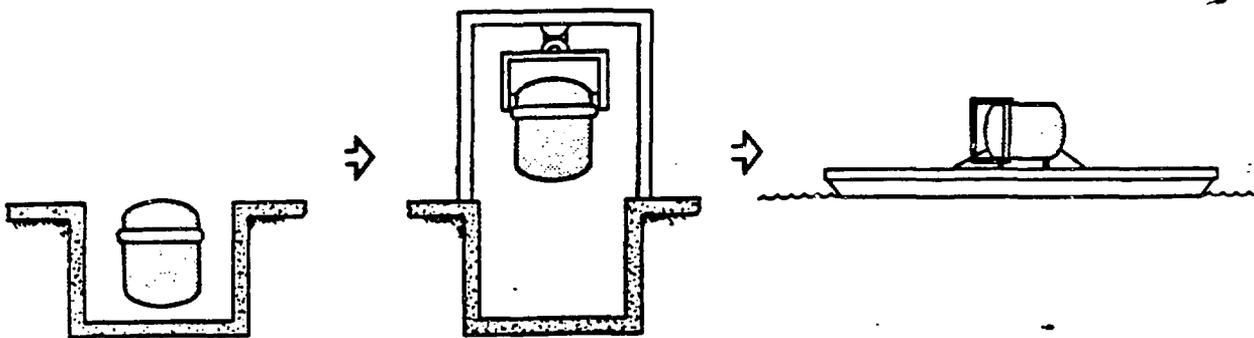
By demonstrating this concept now, utilities may begin to plan to use one-piece removal during decommissioning of their old reactors. Use of this concept will reduce radiation exposure, shorten the project schedule, reduce project costs, and, as shown by the drawing below, greatly reduce the number of waste shipments to disposal sites.
