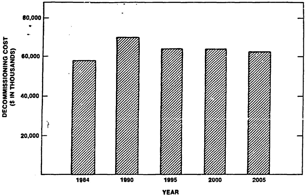
This graph shows that prompt initiation of dismantlement results in lower cost than even a few years delay in the project. For example, dismantlement initiated in 1984 will cost a total of approximately \$60 M, excluding preliminary engineering. Dismantlement initiated in 1990 would result in a total cost of approximately \$70 M in "time value" dollars.
