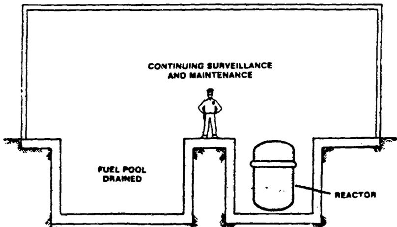
**Entombment is defined as encasement of radioactive materials and components in a massive structure, sufficiently strong and long-lived to ensure the retention of the radioactivity until it decays to unrestricted use levels. During the entombment period, security, surveillance, monitoring, and maintenance are provided.**
